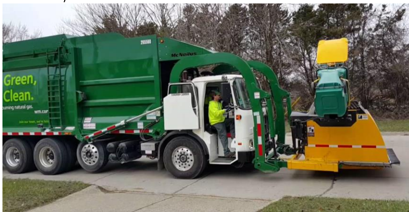
A WM truck equipped with the Auto-Can automated system.
